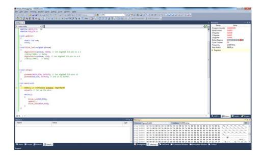
In addition there should be a Breakpoint window showing all the currently set break points, a Processor window showing the values in all the CPU registers (I/O registers are not shown!), and a Watch window showing values of variables. If any of these windows are missing, you can use the View menu to open them.
