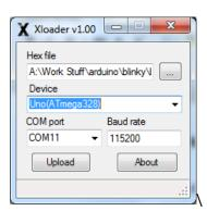
d. Click the "..." button at Hex file, navigate to the directory where the .hex file is, click on the .hex filename, then click Upload. This will upload the file onto the Arduino.
