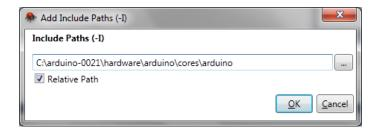
Click OK. Also add in c:\arduino-1.0.1\hardware\arduino\variants\standard.
